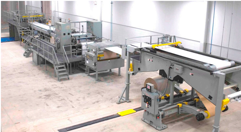
The SheetRunner is a dual-rotary sheeter, optimized for high-volume board production and designed for folding carton plants and commercial printers. (© BW Papersystems)
